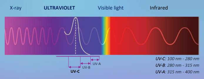
Germicidal ultraviolet (UV-C) radiation - kills microorganism such as bacteria, viruses, mold, fungus and spores that transmit infections, cause allergies, trigger asthma attacks or cause other unhealthy effects. UV destroys the DNA of these microbial contaminants and makes them sterile. UV-C light with a wavelength of 253.7 nanometers is germicidal - i. destroys the DNA of bacteria, viruses and other pathogens, thus destroying their ability to multiply and cause disease.
